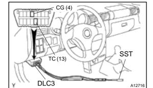
(b) Using SST, connect terminals TC (13) and CG (4) of the DLC3.
